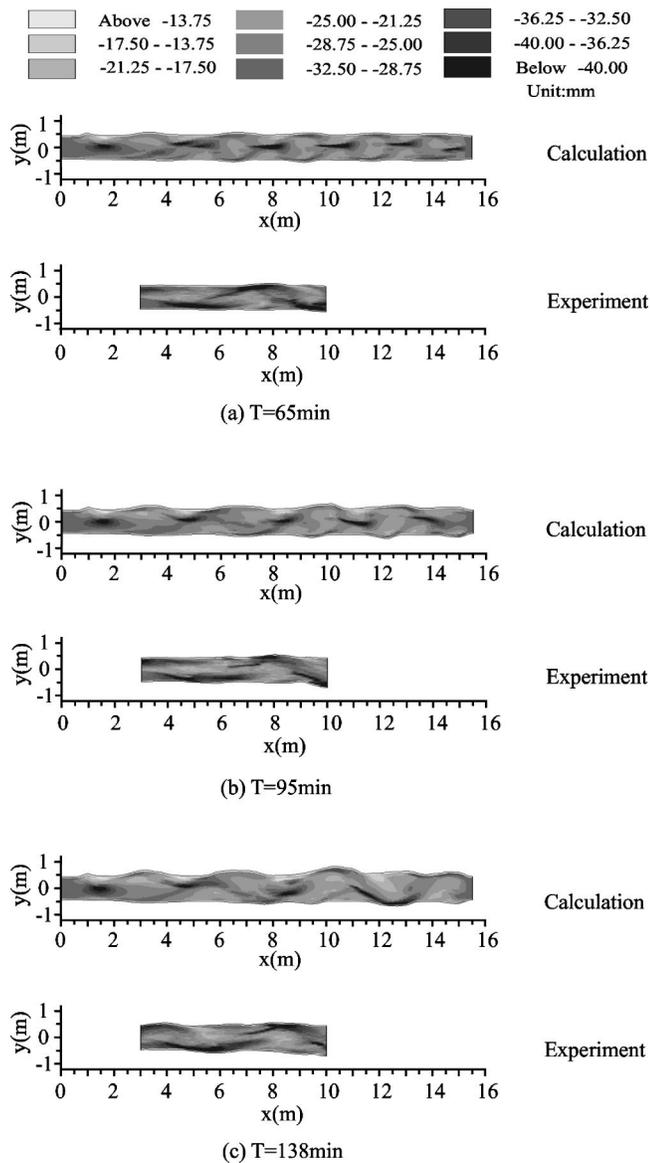
**Fig. 8.** Comparison of channel evolution between numerical and experimental results for Run 1. Flow is from left to right.
