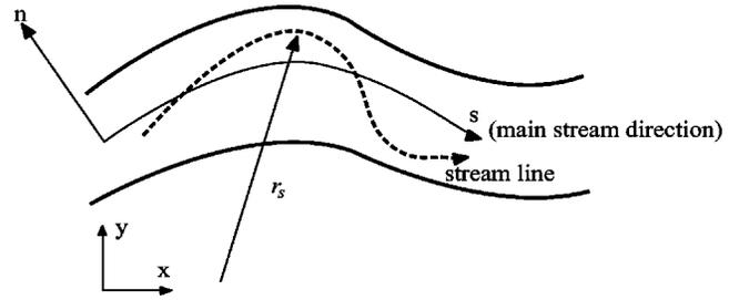
Fig. 2. Definition sketch of stream line and radius of curvature ( $r_s$ )
