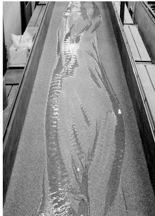
**Fig. 7.** Development from a straight channel into a channel with central bar channel. Experimental result for Run 2 after stopping water flow momentarily. Run time is 95 min. Flow is from top to bottom.
