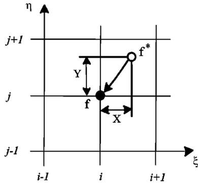
**Fig. 3.** Conceptual diagram of the cubic interpolated pseudoparticle method used in the computational domain
