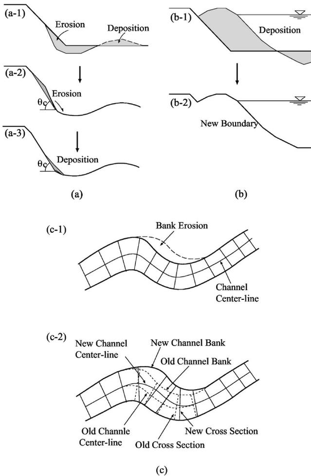
**Fig. 4.** Bed deformation and the renewal of channel geometry: (a) Bed degradation and bank erosion; (b) bed aggradation and bank deposition; and (c) bank deformation and renewal of the computational grid aggradation
