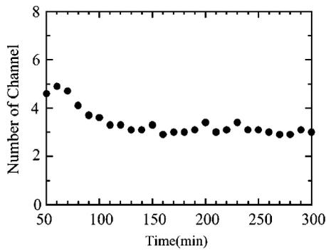
**Fig. 13.** Average number of streams per the width of the braided river with time
