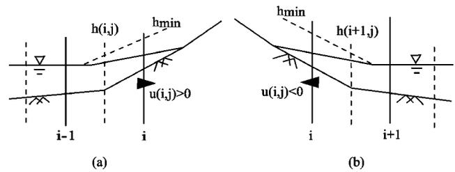
**Fig. 5.** Scheme of boundary near the emerged bars and banks in a staggered grid system: (a)  $dh/d\xi < 0$  and  $u > 0$ , or  $dh/d\eta < 0$  and  $v > 0$  in the longitudinal or transverse direction and (b)  $dh/d\xi > 0$  and  $u < 0$ , or  $dh/d\eta > 0$  and  $v < 0$  in the longitudinal or transverse direction
