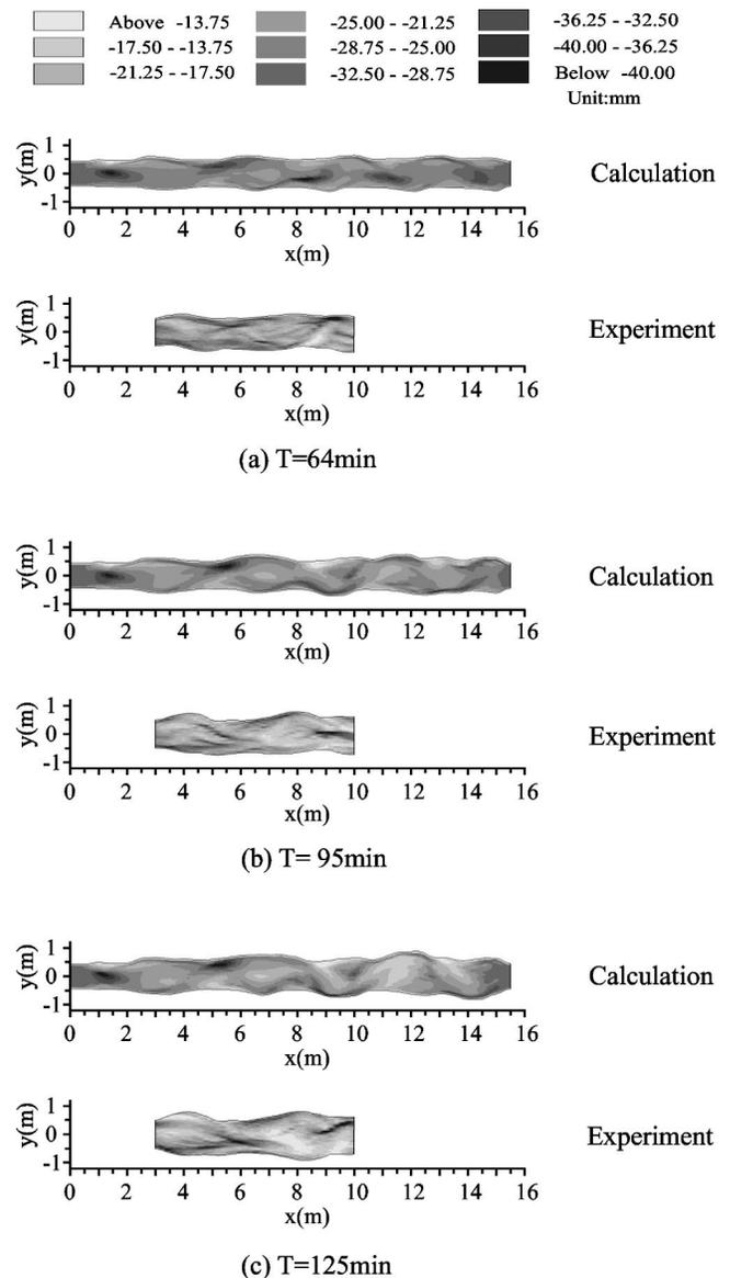
**Fig. 9.** Comparison of channel evolution between numerical and the experimental results for Run 2. Flow is from left to right.
