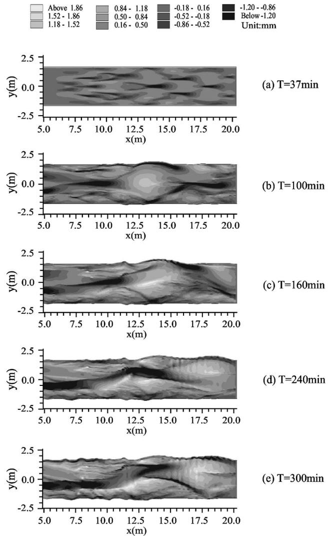
**Fig. 12.** Simulated braided river. Flow is from left to right.
