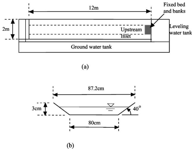
**Fig. 6.** Diagram of experimental setup: (a) Plan view and (b) initial cross section
