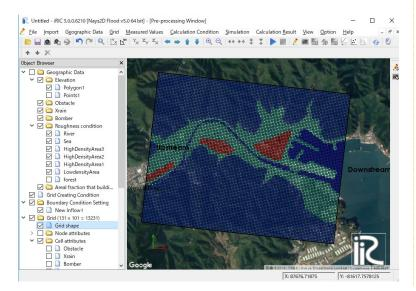
Note: Check whether the roughness coefficients are properly displayed on the grid.
