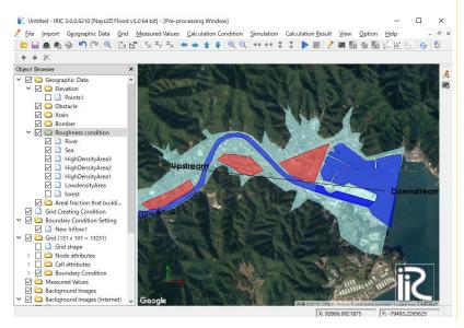
Note: Manning's roughness coefficient is comprehensively set by considering simulation models, land use in the basin and past records. Refer to page 33 of Flood Simulation Manual (Draft) and page 89 of The Collection of Hydraulic Formulae (Japan Society of Civil Engineers (FY 1999).
