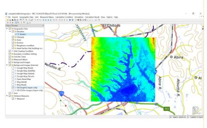
When creating grids for calculation, importing background images such as maps and aerial photos makes it possible to create grids that incorporate riverbanks and land use. Obstacle cells and roughness cells mentioned below can be set in reference to the background image.
