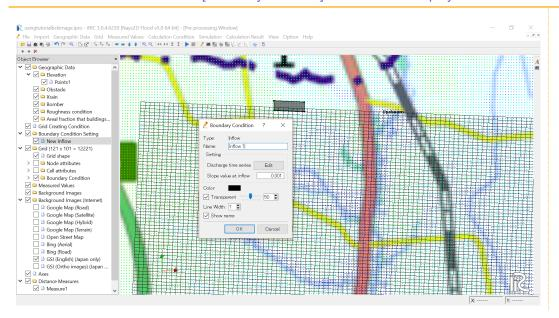
On the [Boundary Condition] window, input "Inflow 1" to the [Name] box, and select [Edit] for the [Discharge time series] box under [Setting].
