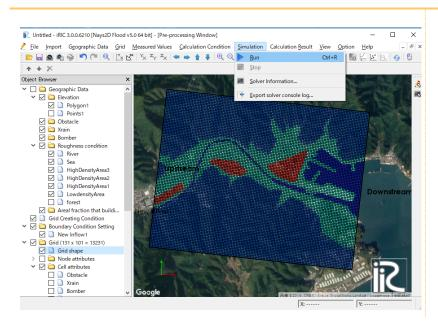
The [Solver Console [Nays2D Flood] (running)] window will open to start the simulation.
