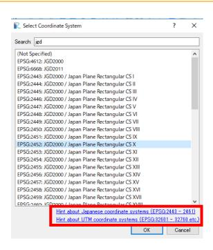
The coordinate system of the target area can be understood from the hint on the coordinate system at the bottom of the screen.
