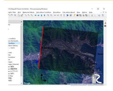
Note: In this basin, an inflow to the mainstream occurs on the red line, as is shown by the blue arrow. Because this sample focuses on tsunami runup, a dummy inflow discharge datum (Discharge 0 m³/s) is applied.
