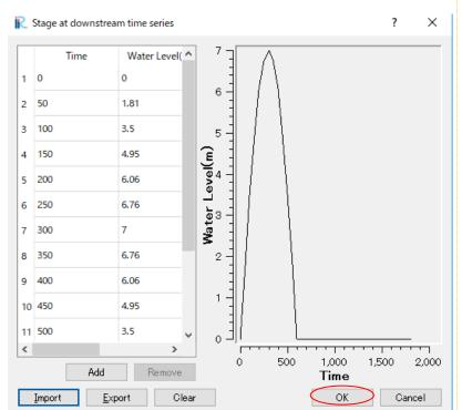
The time steps of the tsunami wave height must be kept at the same value, including at the inflow location.
