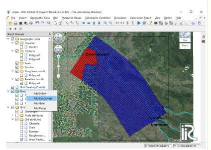
Pass the water through the box culvert to the road set for the obstacle cell.
