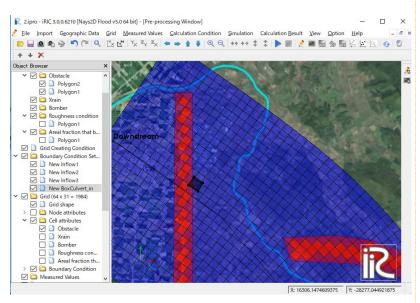
In the figure on the left, the object browser [grid] -[cell attribute] - [obstacle cell] is checked so that the location of the obstacle cell can be seen on the figure.
