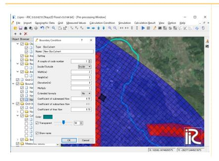
Change the name on [Boundary Condition] screen to [new Box Culvert\_in] and set it as an inside.
