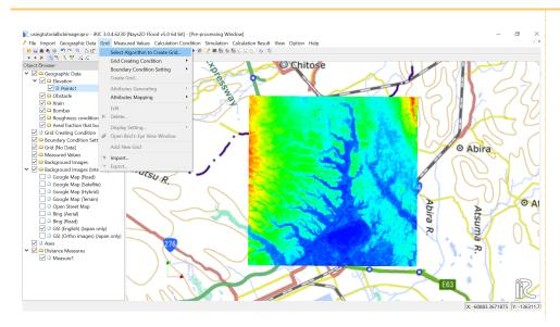
Select [Create grid from polygonal line and width] from the list under the [Select Grid Creating Algorithm] window, and click on [OK].
