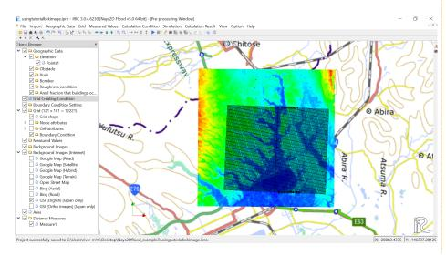
Adjusting the calculation grid
