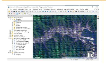
If your PC specifications are insufficient, you may not be able to process very large arrays of elevation data. To speed up processing, remove geographic data in the areas that are not needed.
