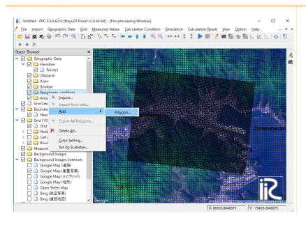
Click on several points to set several vertices such that the vertices enclose the grid area, and press the Enter key on your keyboard to complete the operation.
