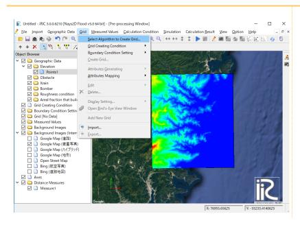
Select [Create grid from polygonal line and width] from the list under the [Select Grid Creating Algorithm] window, and click on [OK].
