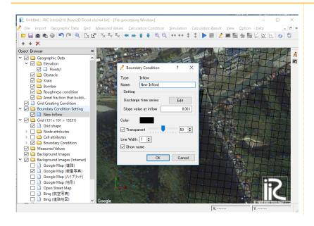
On the [Boundary Condition] window, input "New Inflow 1" to the [Name] box, and select [Edit] for the [Discharge time series] box under [Setting].
