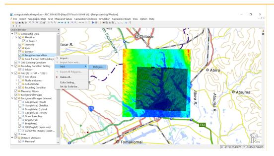
Click on several points to set several vertices such that the vertices enclose the grid area, and press the Enter key on your keyboard to complete the operation.
