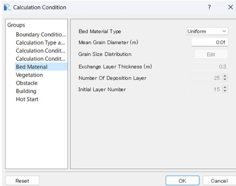
Input mean grain diameter in [Mean Grain Diameter (m)]. This function is available only for uniform sediment
