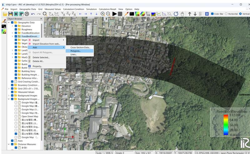
Figure III-2(5) Copy of the fixed bed elevation polygon
