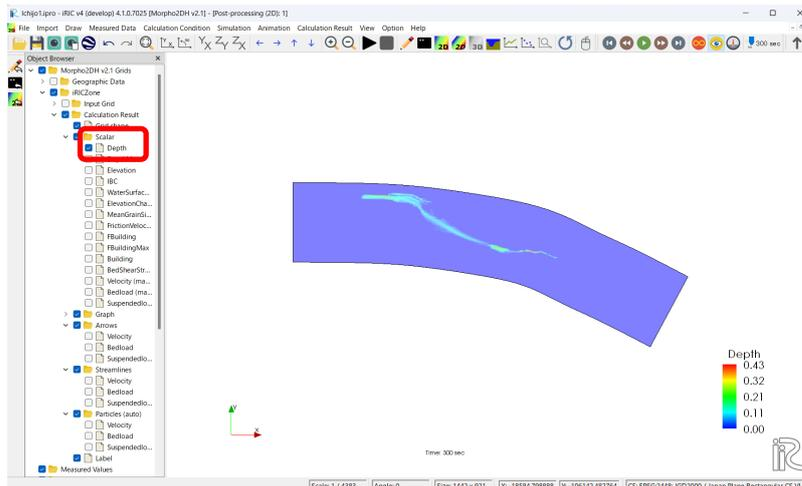
Figure II-10 (2) Make contour of flow depth
