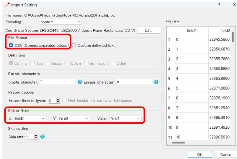
Figure II-4(12) Load the land elevation data
