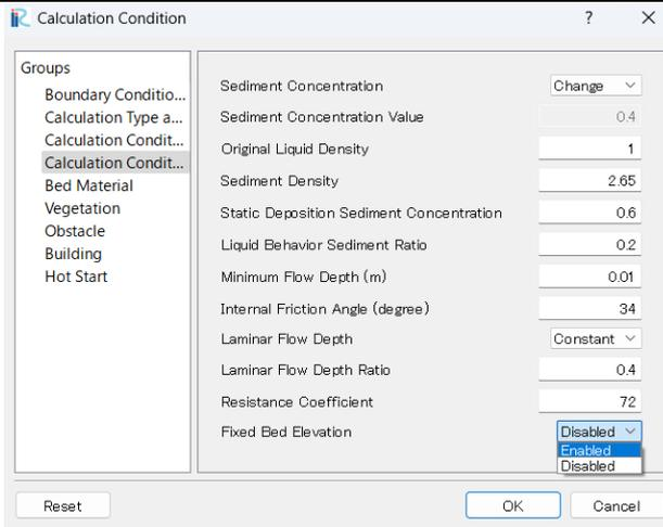
Figure III-3 Enable of fixed bed elevation function
