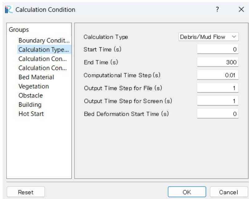
Figure II—8(2) Setting of calculation parameters
