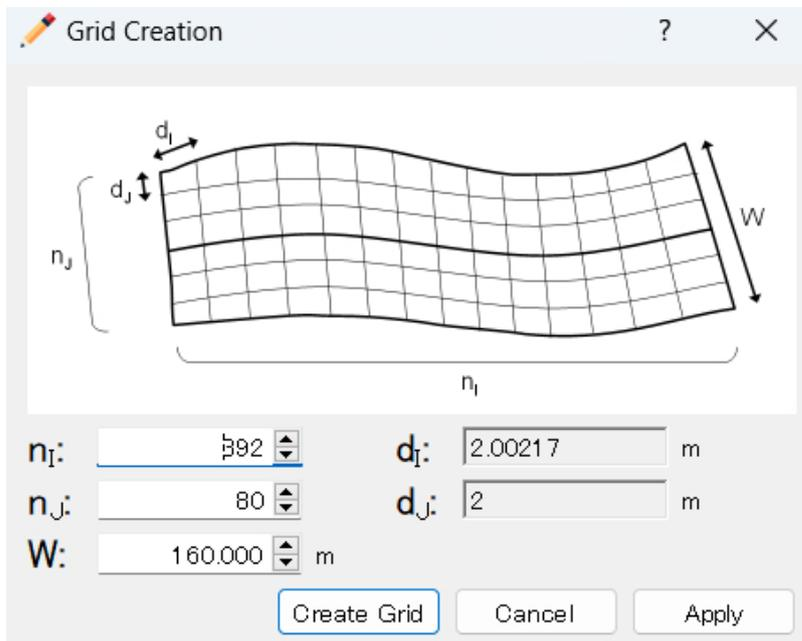
Figure II-4(5) Enter the number of grids, the width of calculation domain.
