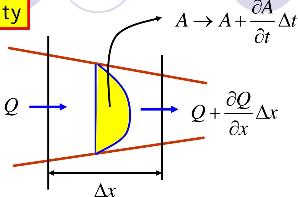
$$\left\{ Q - \left( Q + \frac{\partial Q}{\partial x} \Delta x \right) \right\} \Delta t = \left( A + \frac{\partial A}{\partial t} \Delta t - A \right) \Delta x$$
