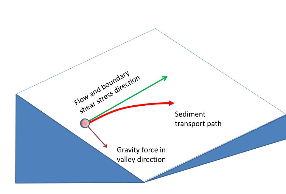
Watanabe et al.[2] proposed the following equation considering the gravitational effect in streamline and transverse directions.
